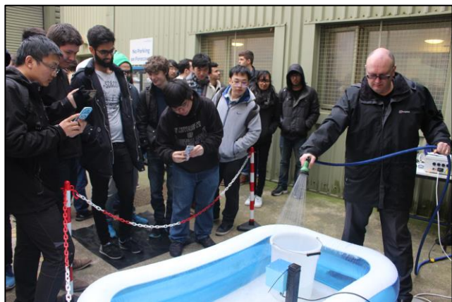
Fig. 2. IP65 testing of the housing.
