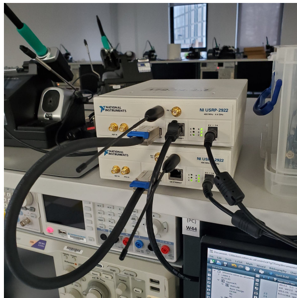
FIGURE 5.1: The setup of two USRP radios. Antennae are connected to both the transmitter (top) and receiver (bottom). A MIMO cable connects the two radios and an ethernet cable connects the transmitter to the PC.
