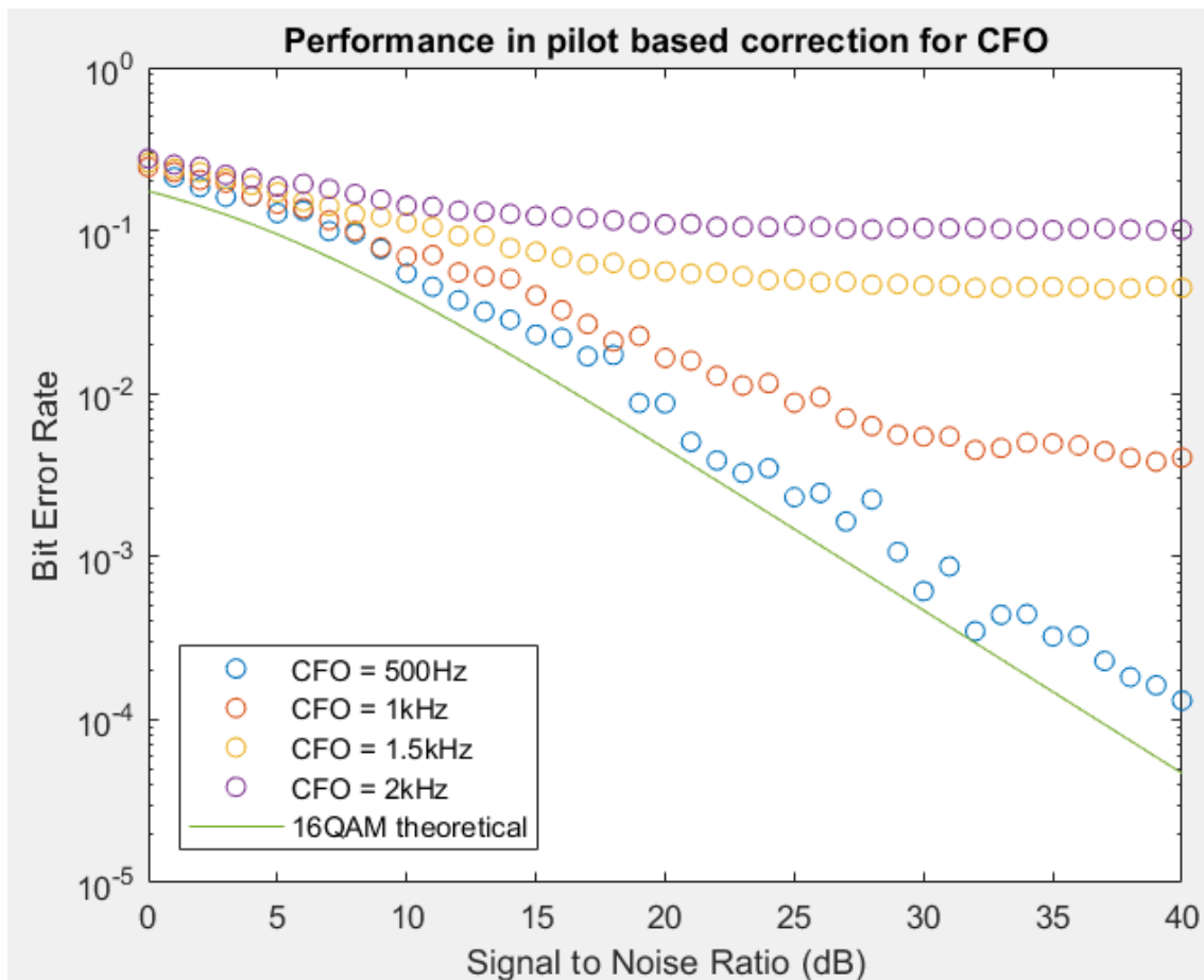
FIGURE F.1: BER in terms of SNR for OFDM system induced with varying CFO
